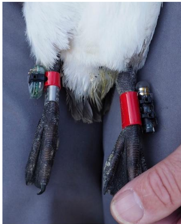
Figure 1. Photo of time-depth recorder (on the left leg) and geolocation-immersion logger (on the right leg, above the metal BTO ring) on a Common Guillemot Uria aalge .
