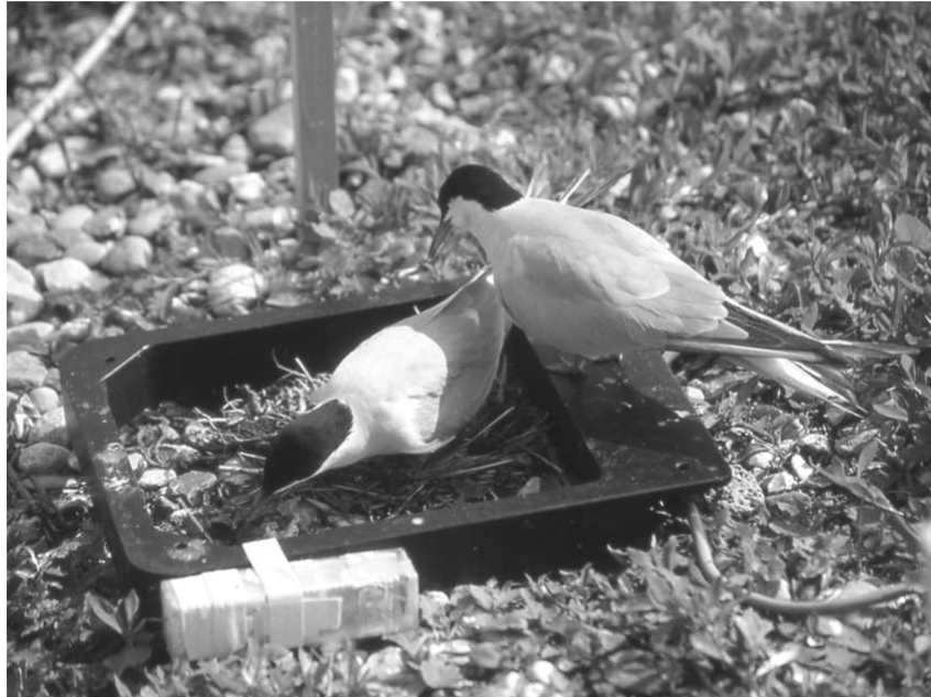
Figure 1. Antenna (black frame) placed around a clutch of a pair of Common Terns within the “Banter See” colony to detect and identify pair mates (the transponder is placed in the breast area of the bird; the part of the body, which is closest to the antenna).
